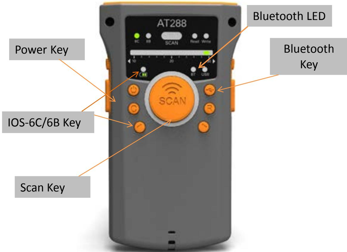
AT288 RFID Scanner must be “Paired” to the tablet prior to scanning Precast items.
