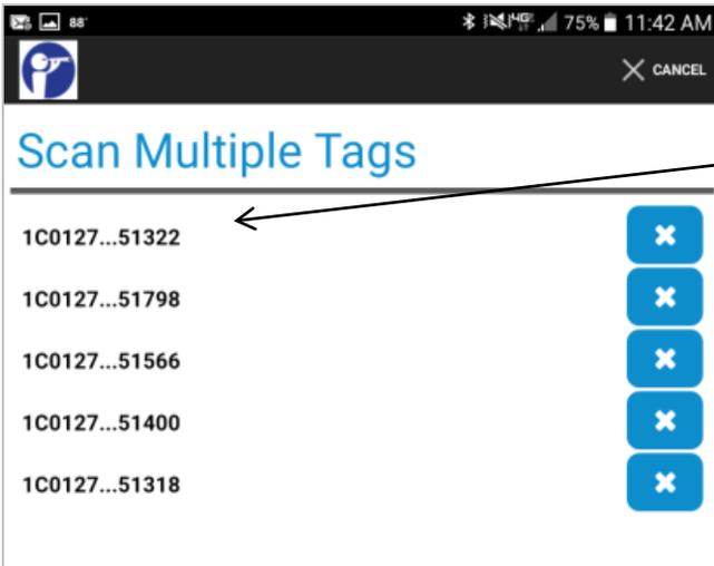
3. To scan the RFID barcode, push the **Scan Key** on the scanner. When the RDIF tag is scanned, the tag numbers appear on the tablets screen.
